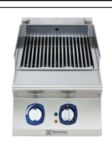
391365 (E9JJCHAOMCG) Half module electric Grill Top HP (high performance). Heating via incoloy armoured heating elements positioned under removable cooking grid, integrated water tap, fixed well with drain, heat boost deflectros,
